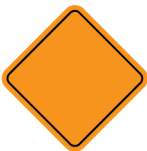
Orange diamond: Construction warning
